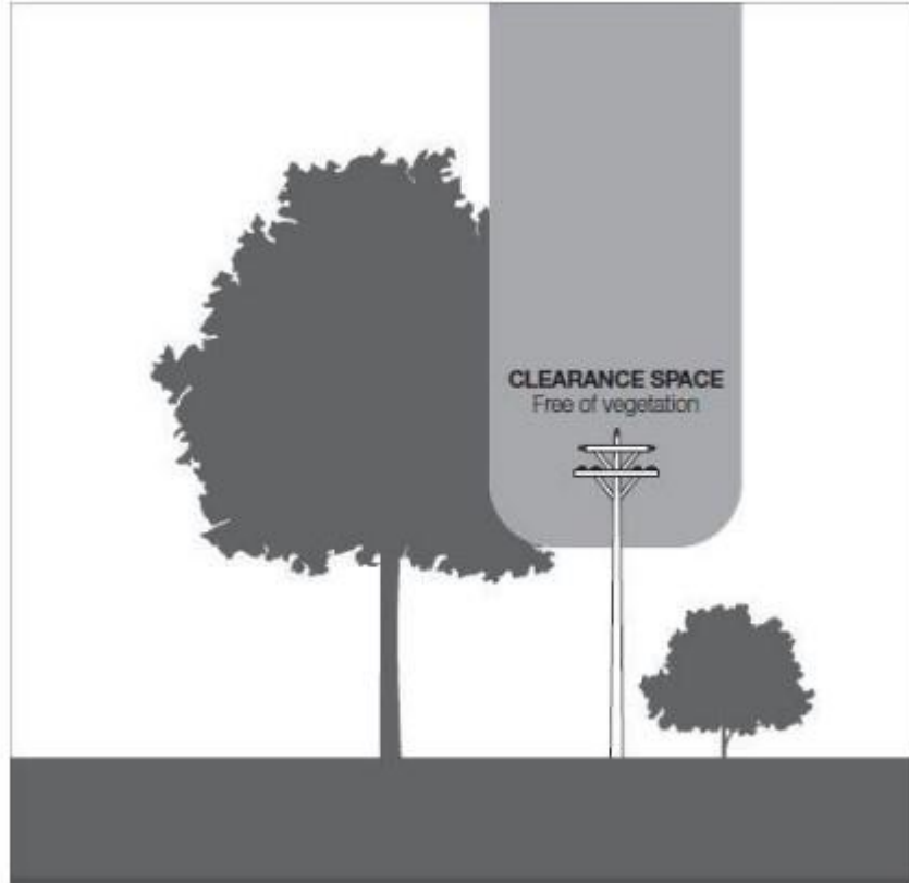
FIGURE 5—UNINSULATED 66 000 VOLT ELECTRIC LINE IN A LOW BUSHFIRE RISK AREA AND UNINSULATED ELECTRIC LINE IN A HAZARDOUS BUSHFIRE RISK AREA
