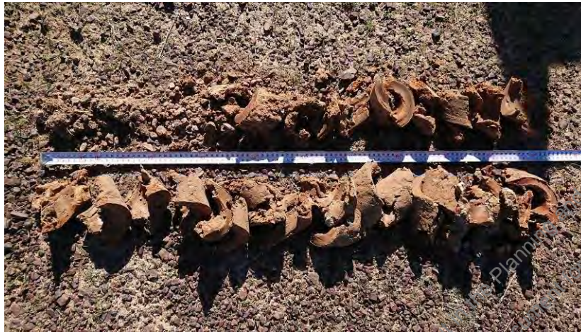
BOREHOLE BH5 (Lot 26): Truncated clay profile from land-soil unit A.
