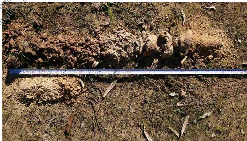
BOREHOLE BH 8 (Lot 4): Typical alluvial profile with alternating sand and clay with indurated zones. Hole terminated at refusal in indurated gravels.
