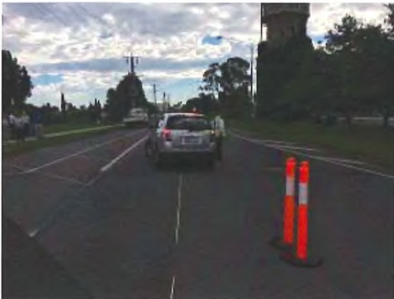
Photo 4: Vehicle undertaking swerving manoeuvre without crossing into the through traffic lane
